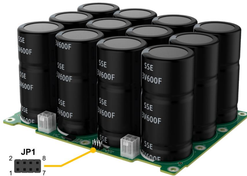
Figure 3-14: Supercapacitor board communication connector Location
