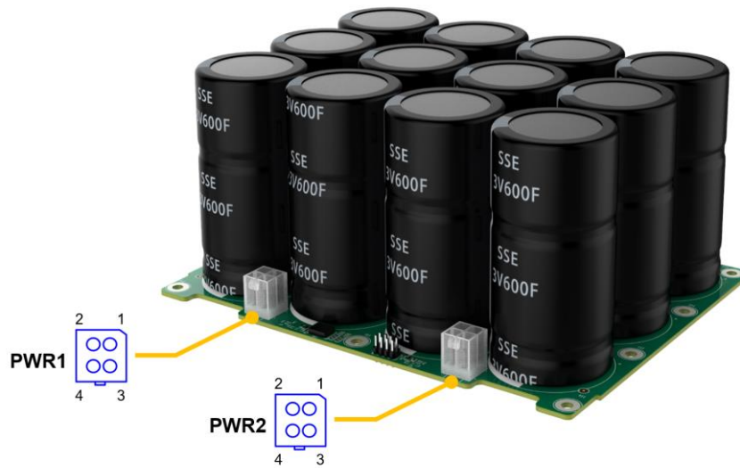
Figure 3-15: Supercapacitor board power connector
