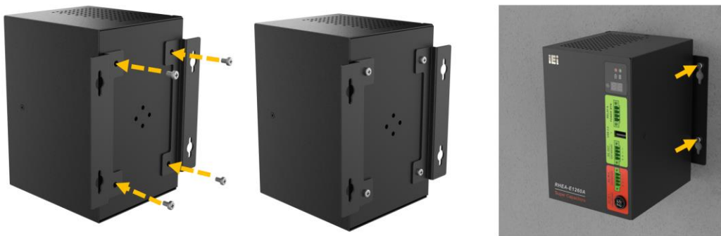
Figure 3-2: Wall mount Installation
